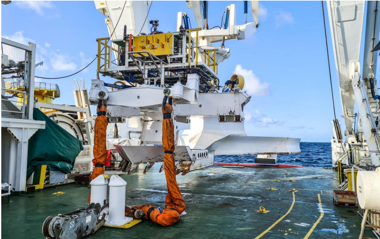
Figure 22: Asso Subsea's Multi-Functional Plough
